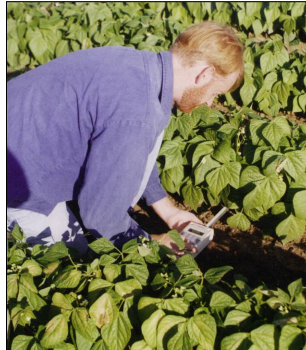
Ground ceptometer leaf-area- index (LAI) measurement
