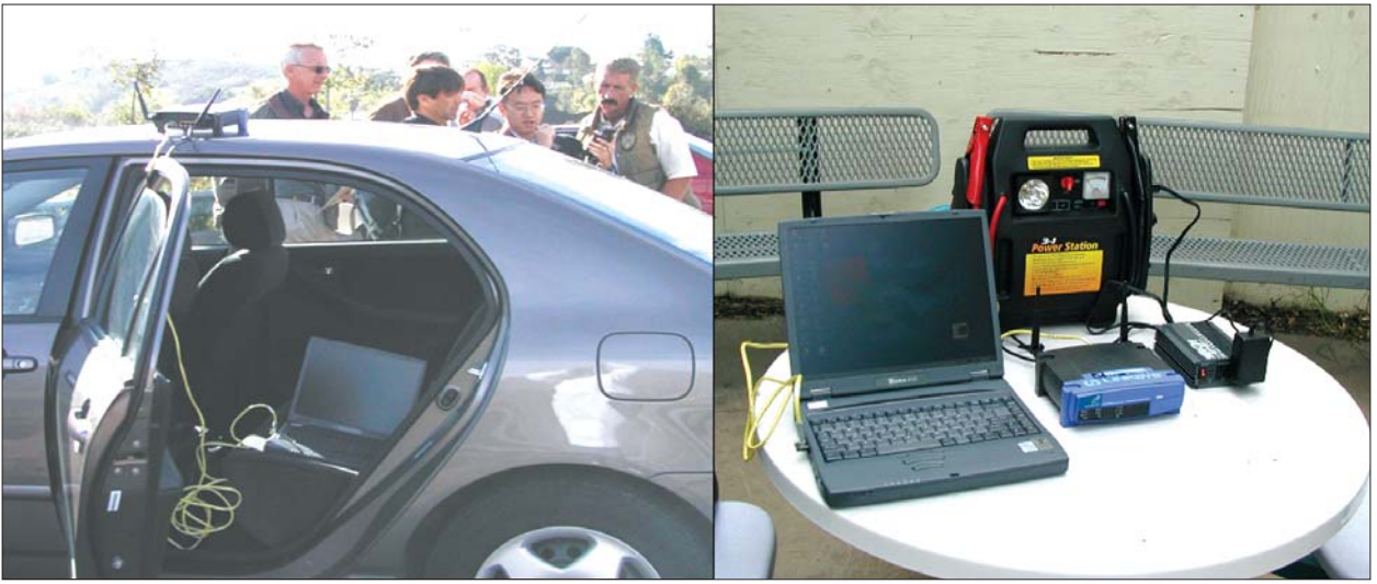
Figure 6. The GIS content server when mounted in a vehicle or connected to a portable power station.
